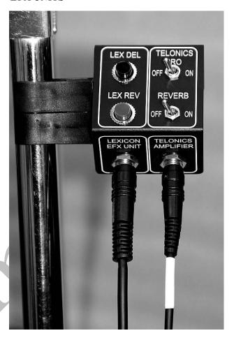
A ¼ inch TRS stereo cable is required to connect the TCA-500B side of the Control Unit to the "Foot Switch" jack on the rear panel of the TCA-500B. This cable is identified by a white ring around the cable directly behind the TRS stereo plugs on both ends. Always be sure the cable with the white ring markings is fully inserted into the bottom right side of the Control Unit, with the TRS stereo plug on the other end plugged into the Foot Switch jack on the rear panel of the TCA-500B.
